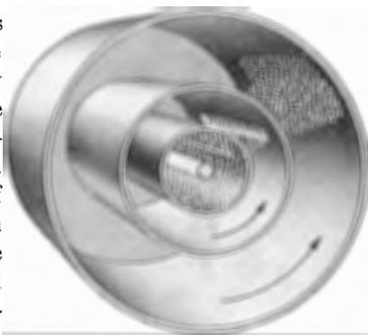
FIG. 20-5. Schematic representation of apparatus for measuring the velocity distribution of gas molecules.
